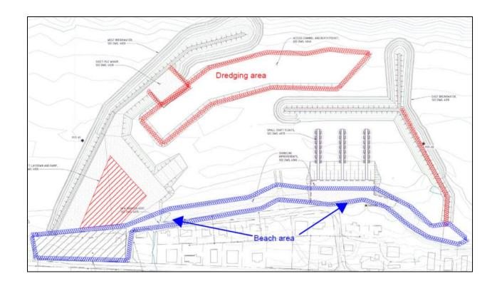
**SAFETY AND ACCESS DURING DREDGING**: During the construction, Tower will phase the construction activities in order to let a fully access to the sealift ramp. **Two lines of buoys will show the path for boats to follow**. **A SIGN WILL BE POSTED** at the beach for information.
